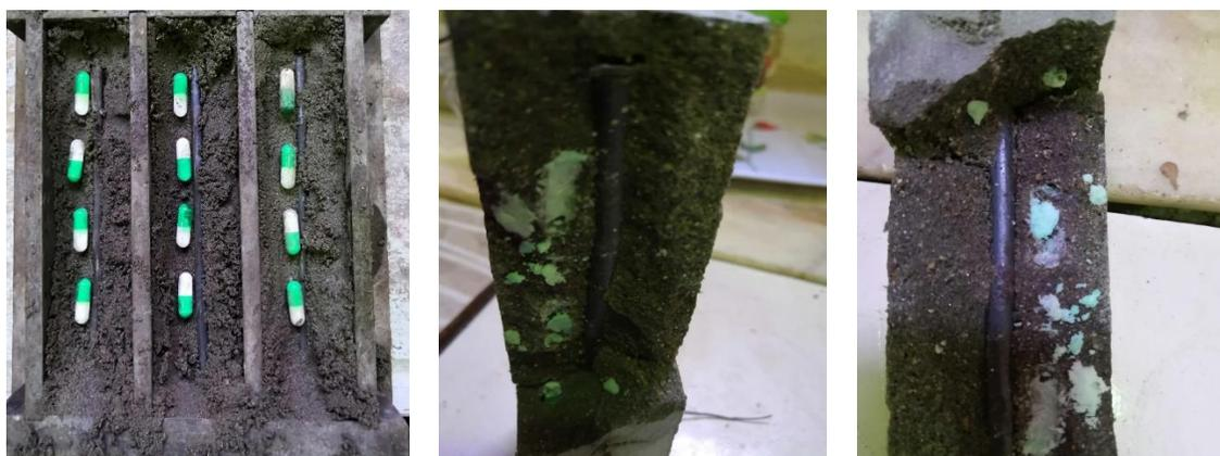
**Figure (1)** Shows Capsulation of Bacterial Spores.
