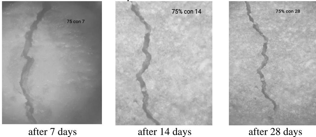
**Figure (6)** Crack healing in the pre-cracked specimens at 7, 14, and 28 days of control specimens at 75 % of maximum load.
