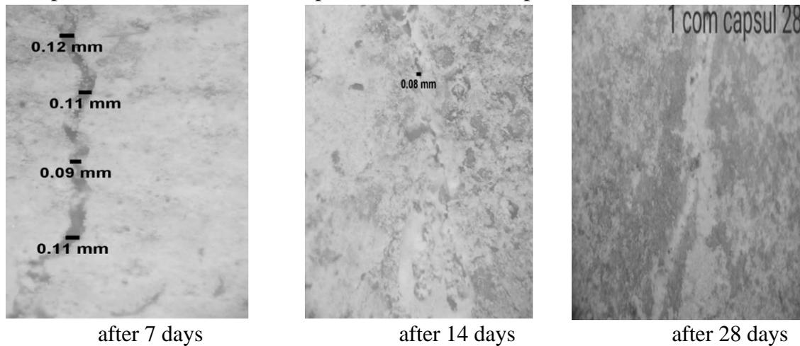
**Figure (11)** Crack healing in the pre-cracked specimens at 7, 14, and 28 days for group (2) specimens which bacterial spores have been encapsulated at maximum load.
