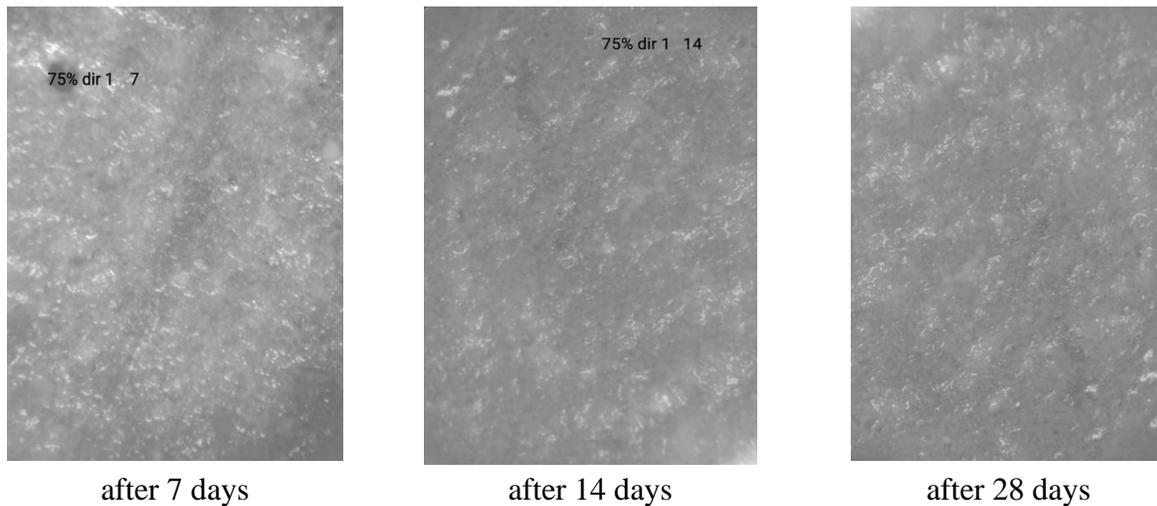
**Figure (8)** Crack healing in the pre-cracked specimens at 7, 14, and 28 days for group (2) bacterial spores were incorporated directly at 75 % of Maximum Load.
