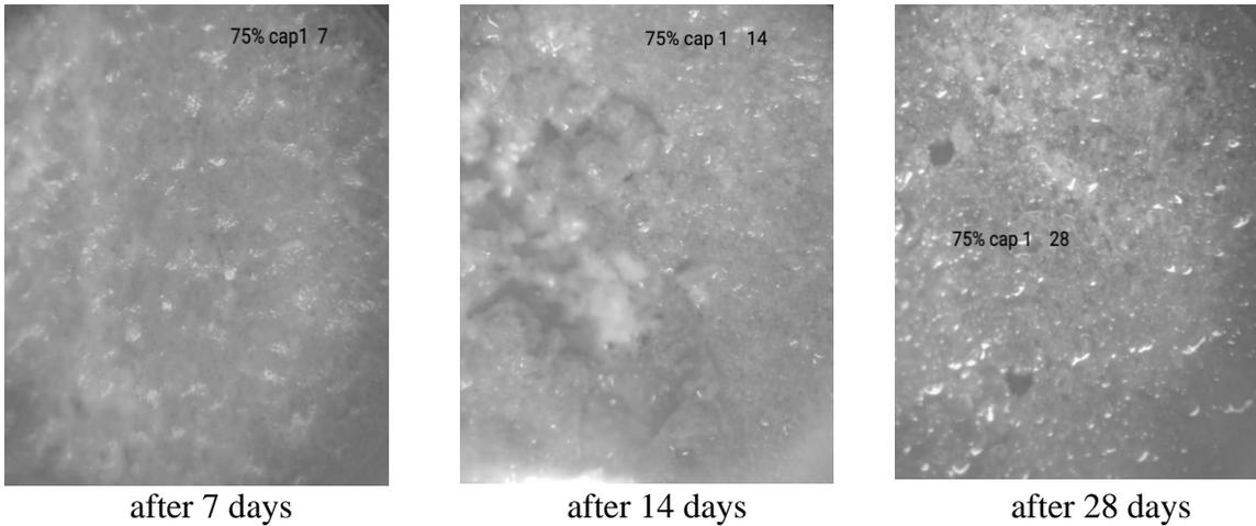
**Figure (10)** Crack healing in the pre-cracked specimens at 7, 14, and 28 days for group (2) specimens which bacterial spores have been encapsulated at 75% of maximum load.
