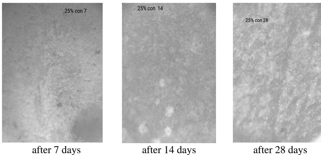
**Figure (4)** Crack healing in the pre-cracked specimens at 7, 14, and 28 days of control specimens at 25% of maximum load.
