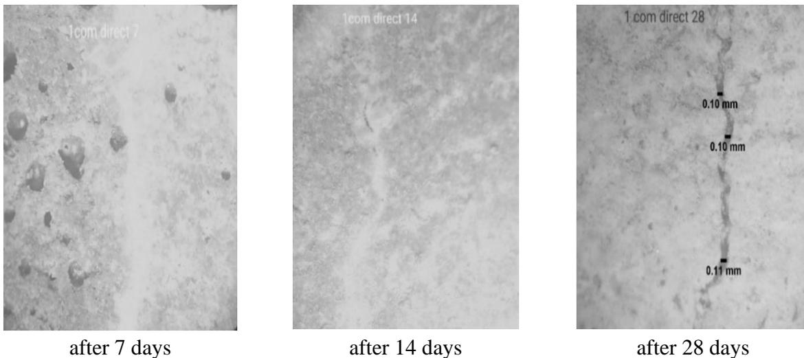
**Figure (9)** Crack healing in the pre-cracked specimens at 7, 14, and 28 days for group (2) bacterial spores were incorporated directly at Maximum Load.
