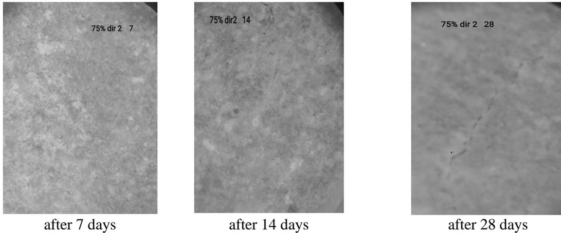
**Figure (12)** Crack Healing in The Pre-Cracked Specimens at 7, 14, And 28 Days for Group (3) Bacteria Were Incorporated Directly at 75 % of the maximum load.
