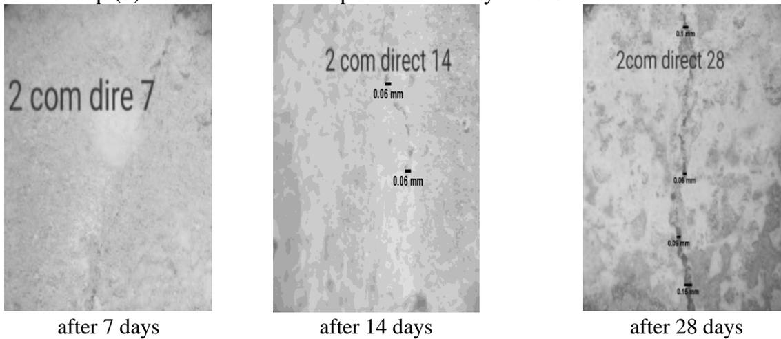
**Figure (13)** Crack Healing in The Pre-Cracked Specimens at 7, 14, And 28 Days for Group (3) Bacteria Were Incorporated Directly at maximum load.
