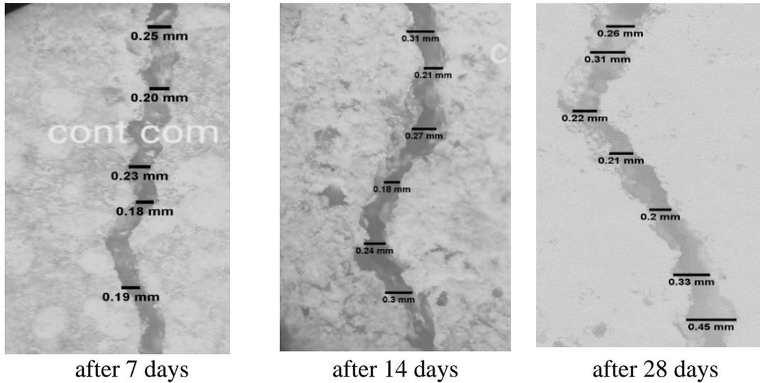
**Figure (5)** Crack healing in the pre-cracked specimens at 7, 14, and 28 days of control specimens at maximum load.
