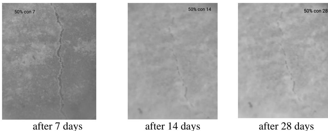
**Figure (7)** Crack healing in the pre-cracked specimens at 7, 14, and 28 days of control specimens at 50% of maximum load.
