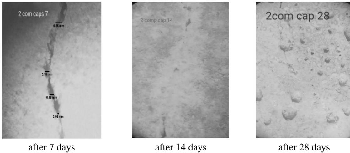
**Figure (15)** Crack Healing in The Pre-Cracked Specimens at 7, 14, And 28 Days for Group (3) Specimens which bacterial spores have been encapsulated at maximum load.
