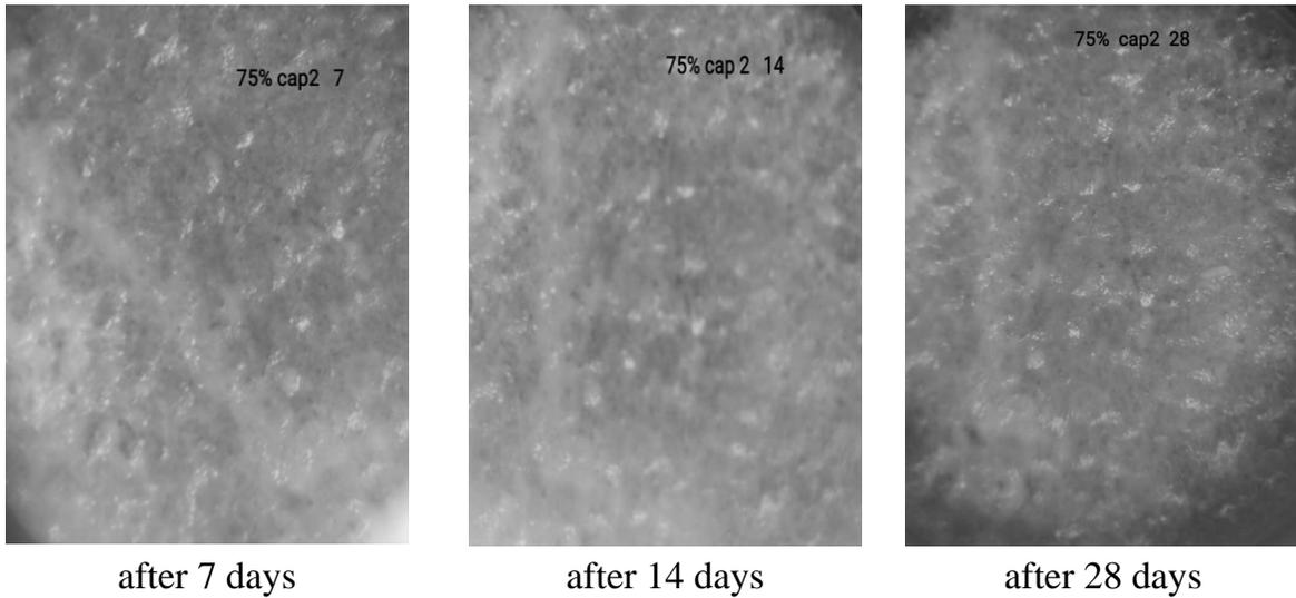
**Figure (14)** Crack Healing in The Pre-Cracked Specimens at 7, 14, And 28 Days for Group (3) Specimens which bacterial spores have been encapsulated at 75% of maximum load.
