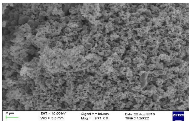
**Figure 1** : Scanning electron micrograph of copper nanoparticles
