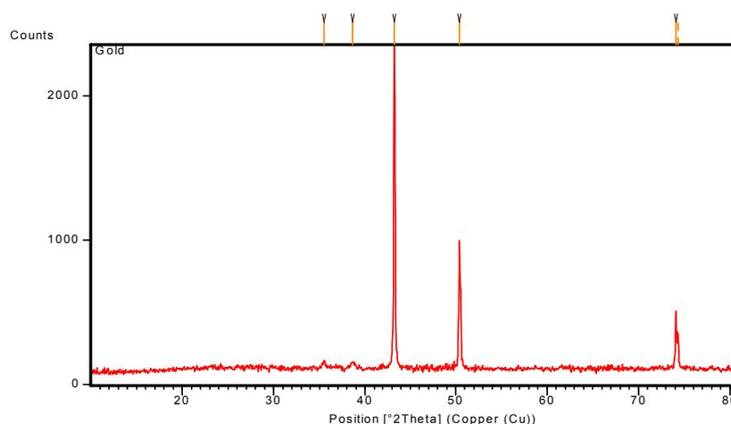
**Fig. 3:** XRD of copper nanoparticles.
