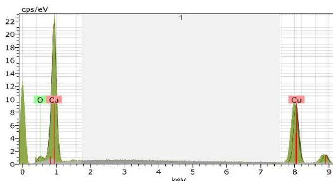
**Figure 2** : Energy dispersive spectrum of copper nanoparticles
