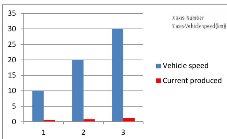
When the speed of the cycle is increased from 10 to 20 km/hr the produced electricity also increases. But the produced electricity was responding very slowly to the speed was revealed from the Graph.I. When the speed of vehicle is 30 km the electricity produced was mere 1.8 volt. Therefore my research shifted towards higher mode of vehicle that is Moped Bike. Dynamo of bike also cannot be used since the speed of bicycle never be raised beyond 30 km speed.
