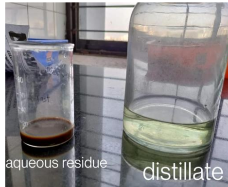
Figure 2: Distillate and aqueous residue are separate filtration and distillation
