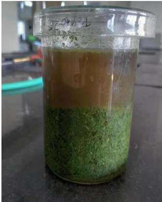
Figure 1: Fermentation of pulverised neem leaves and cream urine
