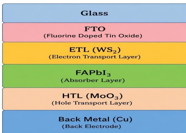
Fig. 1 Configuration of FTO/WS 2 /FAPbI 3 /MoO 3 /Cu perovskite solar cell
