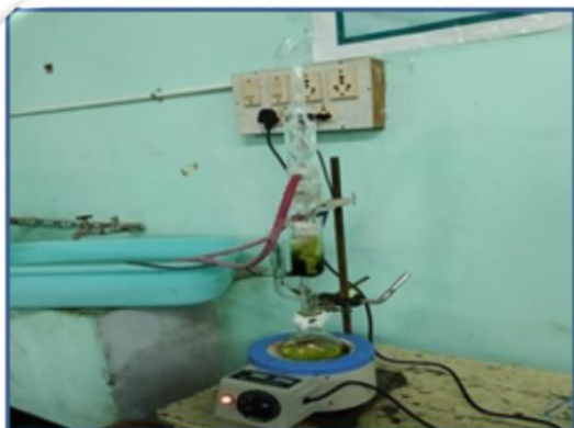
Fig.1. Leaf Extraction Using Soxhlet Apparatus
