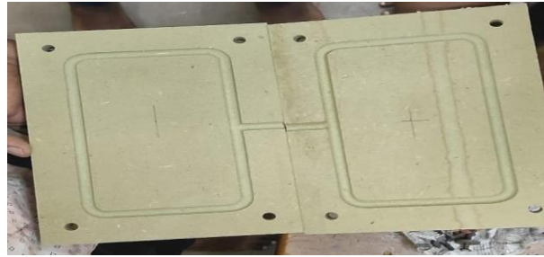
Figure 3 Mould for CGFRP Stirrups
