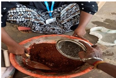
Figure 4 Mixing of clay soil & red soil with Waste stainless steel slag
