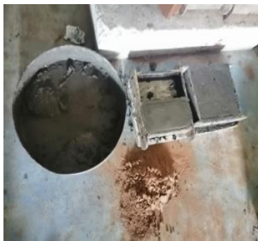
Figure 3 Type 3- Cement Brick (1:2) (1 Part cement 2 Part FA)
