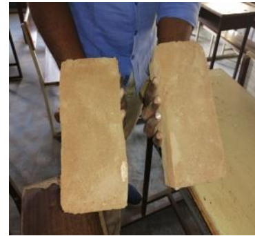
Figure 2 Type 2-Red Soil + Cement (1:3) 25% of cement + 75% of soil
