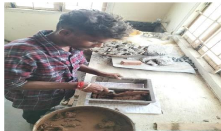
Figure 5 Preparation of making the brick on mould
