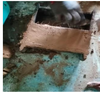
Figure 4 Type 4 -Coir Pith + Soil Bricks (1:100) 10g of coir for 1Kg of soil
