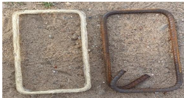
Figure 5 (b) CGFRP Stirrups 8 mm and steel stirrups 8 mm
