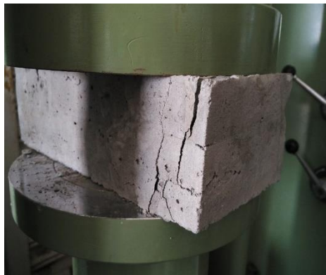
Figure 2 Compression Test on Brick
