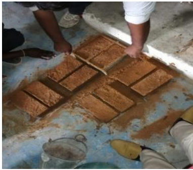
Figure1 Type 1-Red Soil+Sand (3:2) 60% of Soil 40% of Fine Aggregate
